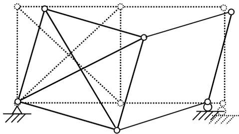
The structure displaces without any members deforming.
