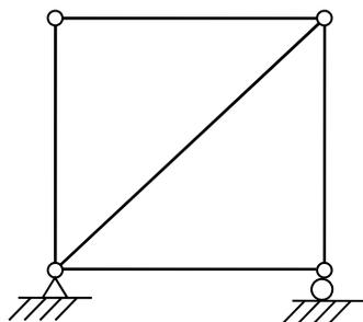
Figure 2a. Stable & Determinate Truss
