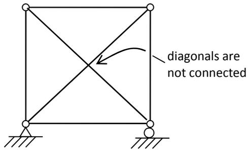
Figure 3a. Stable &amp; Indeterminate Truss
